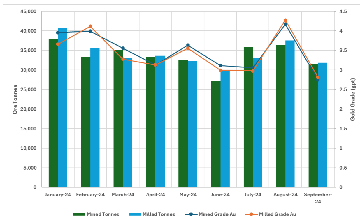
Figure 16-13: 2024 Mine versus Mill tonnes and grade
