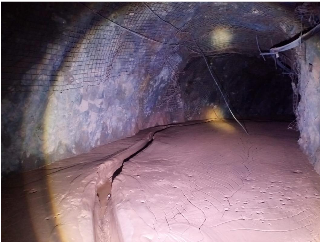
Figure 18-12: Deposited tailings CDO level 930
